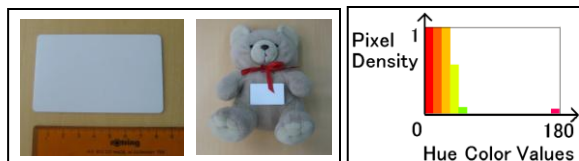
(a) RFID tag put on an object. (b) Its color histogram.
